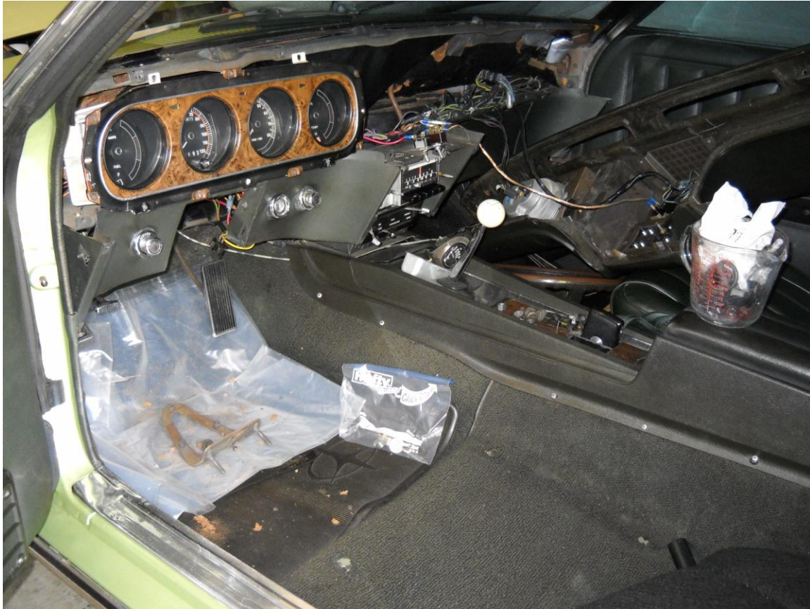
Interior with driver's seat, steering column, dash pad removed. Note plastic liner to protect carpet. The bracket on the floor mounts behind the instrument panel to the dash structure and provides anchorage for the steering column mounting studs seen in the bracket. Brake booster studs are now easily accessible through steering column and instrument cluster voids.
