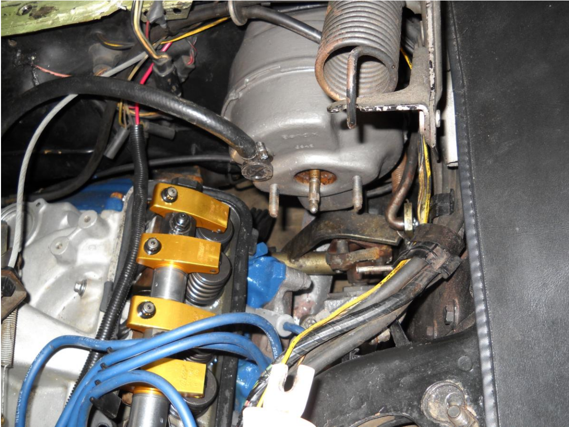
Export Brace, Monte Carlo Bar, Valve Cover and Brake Master Cylinder removed. Steering column to steering box attaching nuts exposed just below top of Z-bar. The retaining pin for the through the dash rod is now easy to access.
