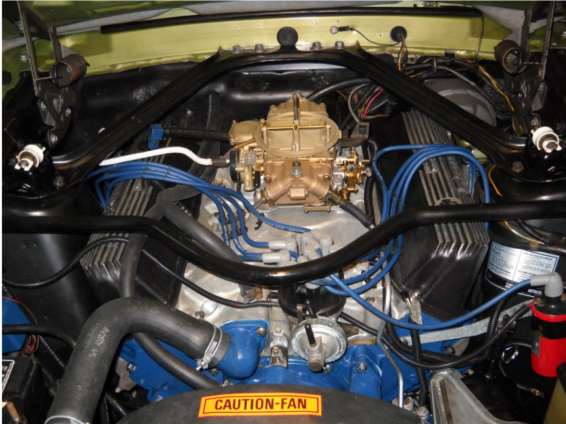
Engine compartment showing Export brace and Monte Carlo bar that must be removed to remove driver side valve cover for brake booster removal. Note torque strap bolted to driver's side cylinder head and fender well and relocated coil to reduce coil heating. Aluminum manifold is a 427 K-code medium riser port matched to the 428CJ heads. Carburetor is a numbers correct 735 CFM Holley.
