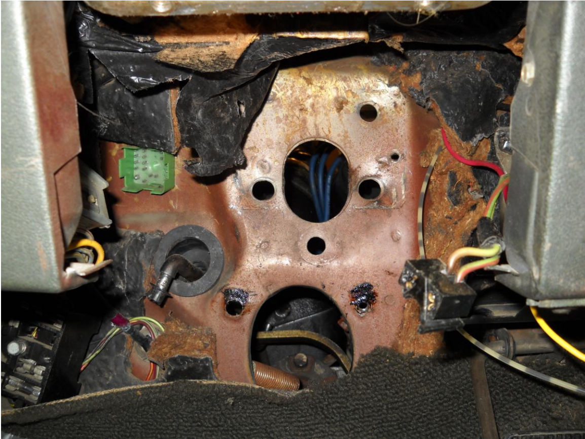
Brake booster and steering column holes through fire wall after pedal bracket removal. Some insulation repair is needed before reassembly. Fuse box was removed from firewall to avoid damaging it. This does not need to be done if the steering column is out.
