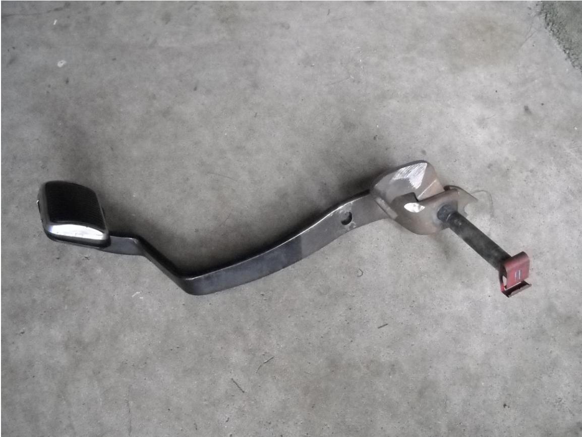
Original clutch pedal. Note cut in pedal shaft near pedal where pedal bracket wore into shaft and oval shaped rod hole necessitating pedal repair or replacement. Wear on pedal was the result of pedal play from worn pedal bearing and shaft.
