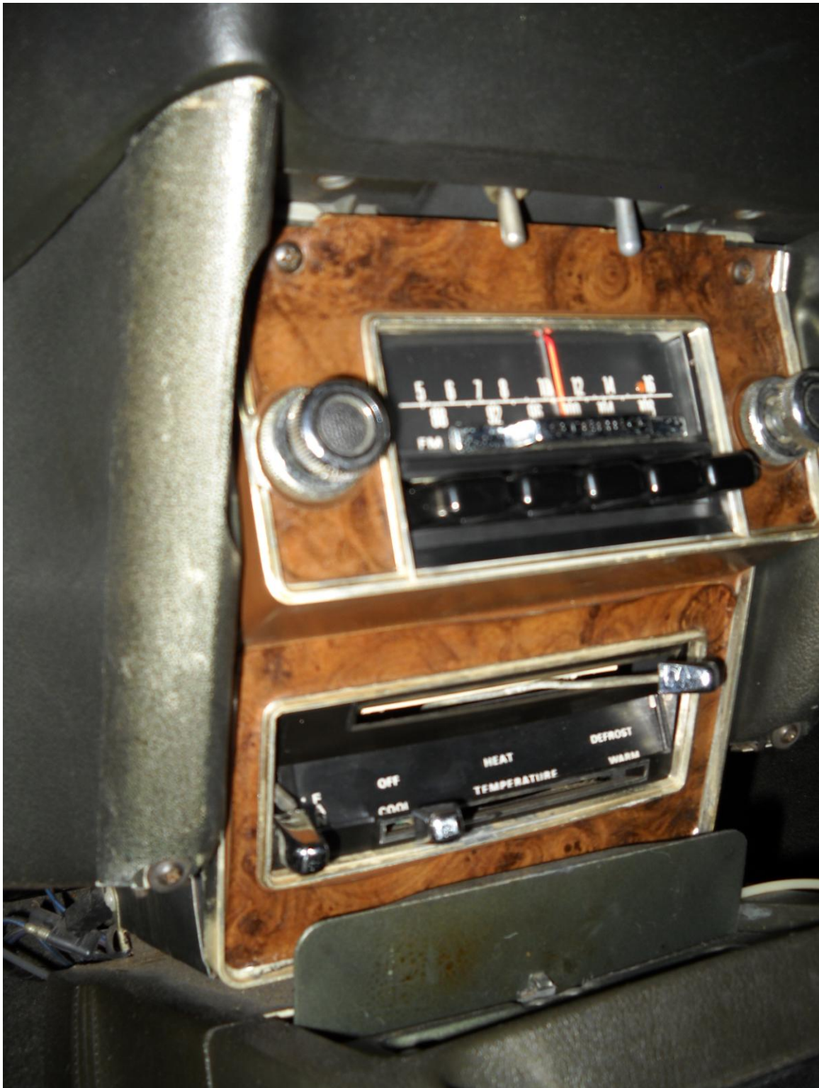
Radio/heater trim panel that must be removed to access trim and dash attaching screws. Note two Philips head screws at top of trim piece.
